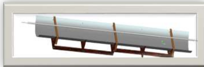
Figure1: Solar Parabolic Trough Collector Assembly
